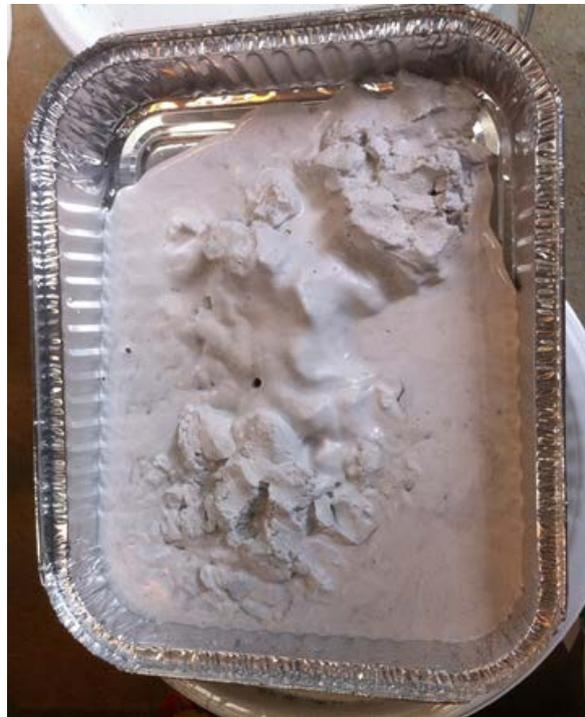
Figure I.30: Product cenospheres obtained from the multi-stage IRC™ process.
