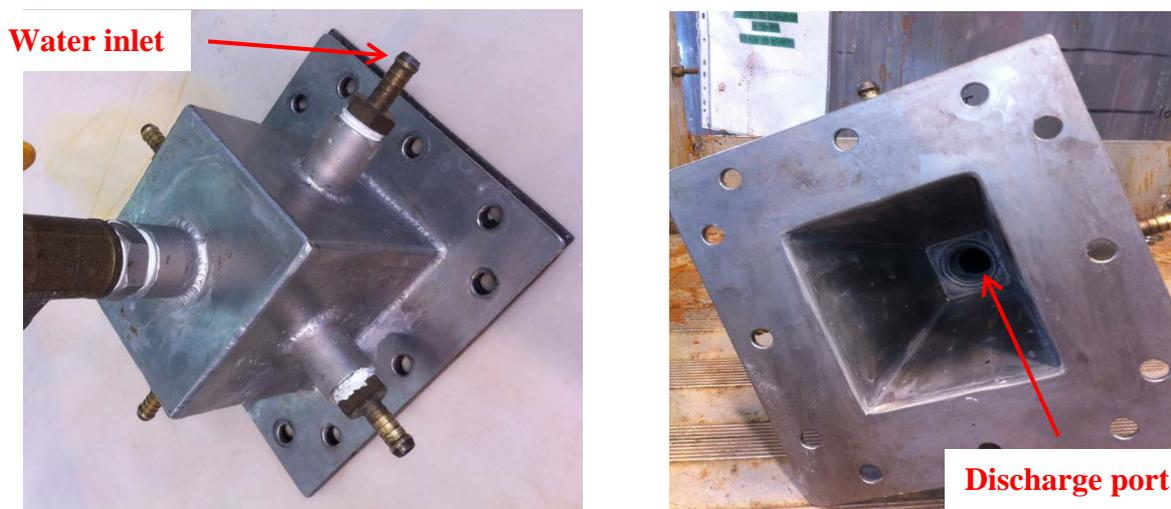
Figure 5.2: The fluidization water distributor with 4 water inlets to the chamber and 14 holes in each face of the distributor.
