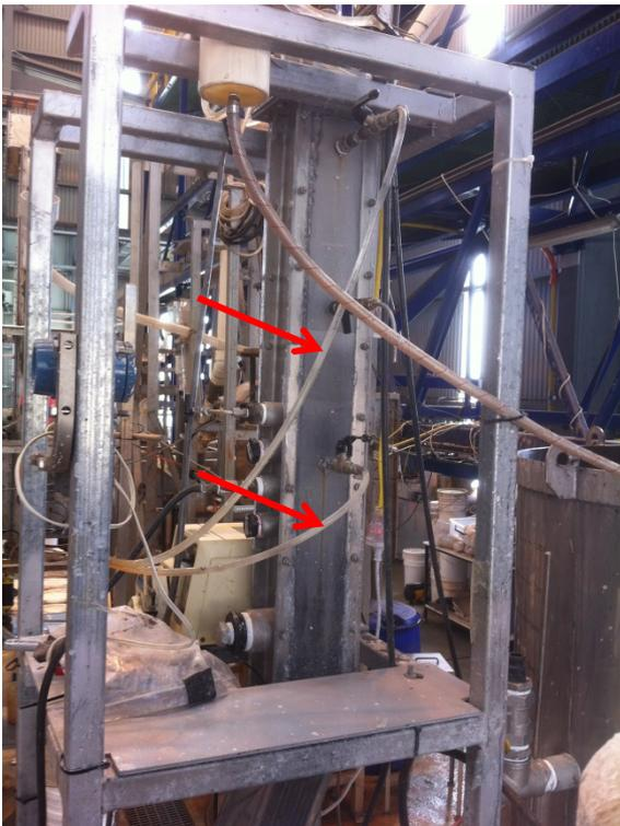
Figure I.5: The pressure transducer tubes.
