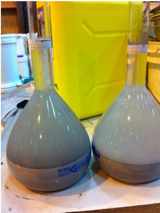
Figure I.29: Fly ash and cenospheres volume fraction comparison between two tanks used in the pilot runs.
