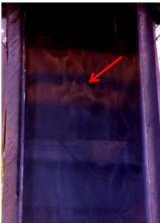
Figure I.19: The white streams developed within the inclined channel near the vertical section.
