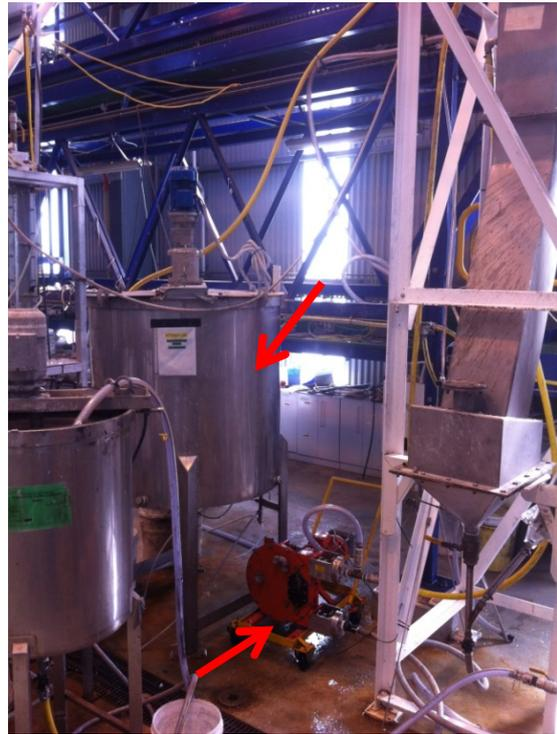
Figure I.24: The feed tank and feed pump used in the pilot scale runs.
