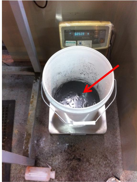
Figure I.16: Black porous particles floated in a fresh fly ash-water mixture.
